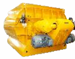
MHW Hazardous Waste Treatment Mixer
